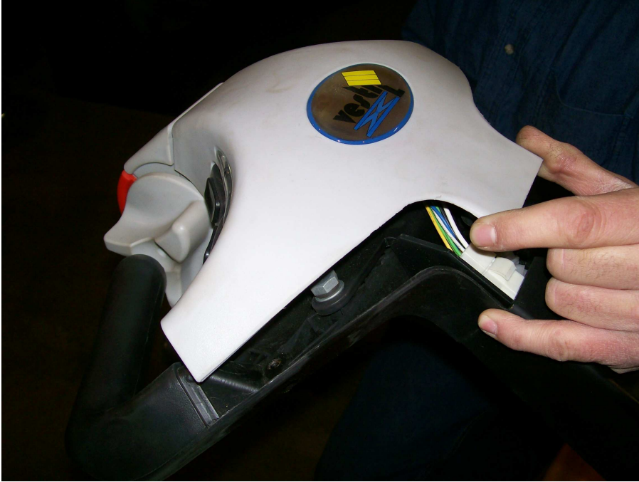
Carefully pull the belly switch back off of the tiller while tipping the front up. Fig 8
